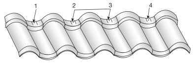
Make sure nose of panel is pulled flush and tight with panel below.
