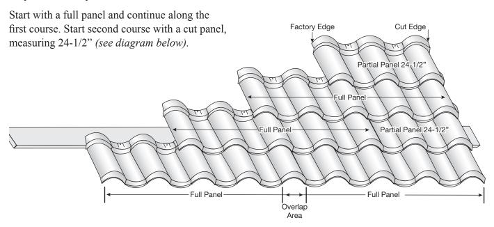
Measure panels and make cuts accordingly so the cut edge starts (or terminates) in the DECRA Channel or Villa Valley (see diagram below). Panels can be cut from either side (see diagram right). Save cut-off pieces for use on opposite side terminating into Villa Valley or DECRA Channel.
