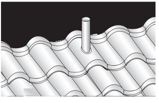
Do not use LEAD or COPPER with this steel roofing system.
