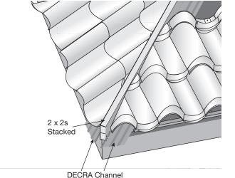
Pre-paint vertical/exposed portion of DECRA Channel & Valley prior to installing panels.
